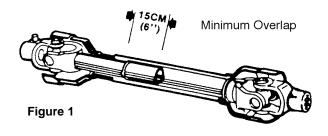
If driveline must be cut to a shorter length, clamp driveline in a well padded vise to prevent damage to the shield. Cut off shield where marked. Using cut-off section of shield as a guide, cut shaft the same amount. (Figure 2)
